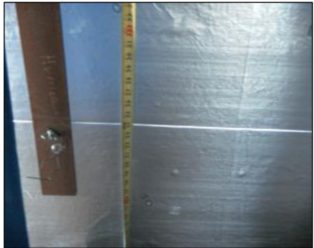
Photo No 99 Post-test, Sliver Perforation Specimen 12
