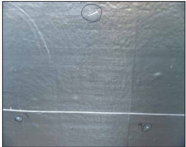
Photo No 86 Post-test, Sliver Perforation and Fragment Indent Specimen 10
