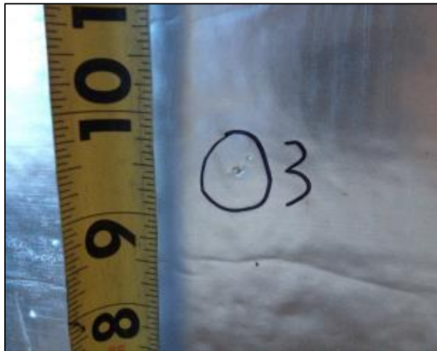
Photo No 48 Post-test, Sliver Perforation Specimen 4
