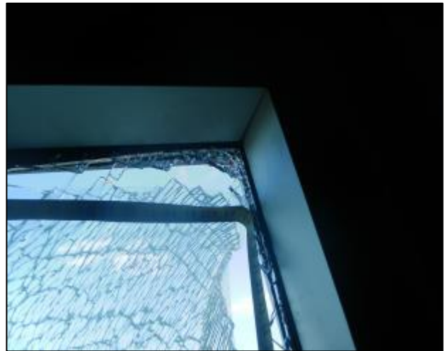
Photo No 179 Post-test, Glazing Tears Specimen 24
