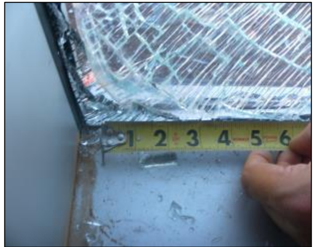
Photo No 183 Post-test, Glazing Tears Specimen 24
