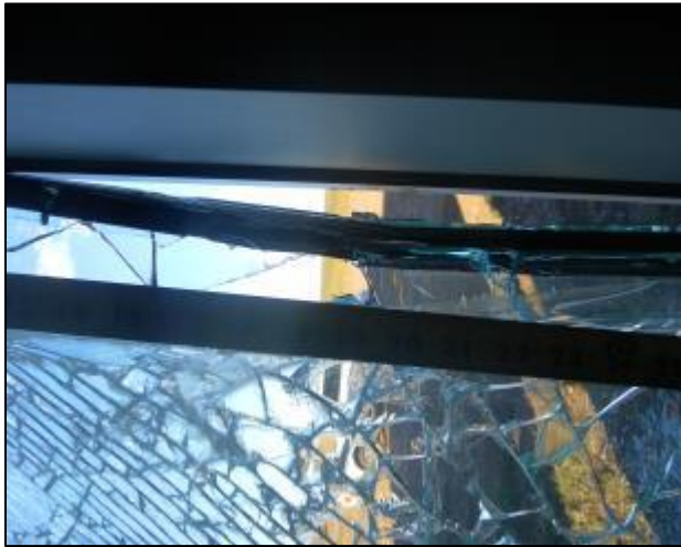
Photo No 180 Post-test, Glazing Tears Specimen 24
