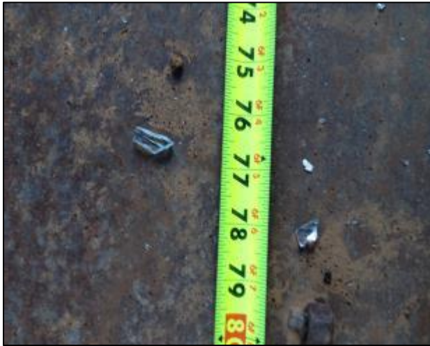
Photo No 18 Post-test, Fragments Specimen 2
