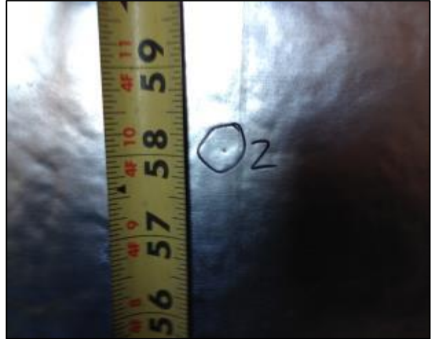
Photo No 47 Post-test, Sliver Perforation Specimen 4
