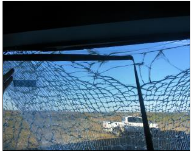
Photo No 177 Post-test, Glazing Tears Specimen 24
