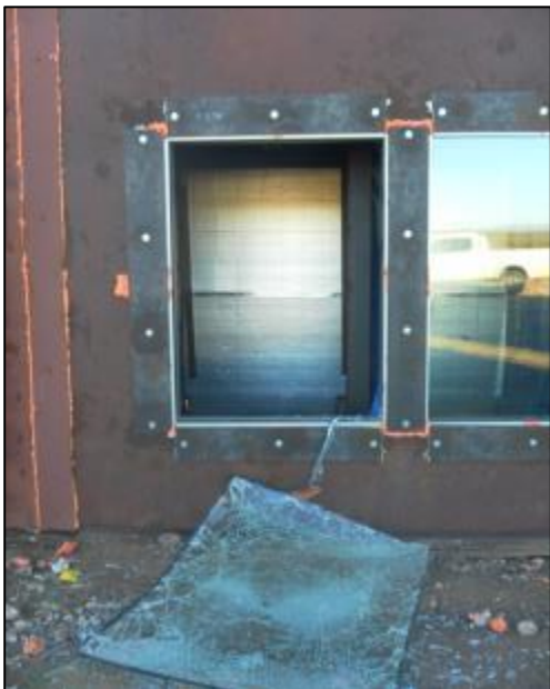
Photo No 155 Post-test, Exterior Specimen 21
