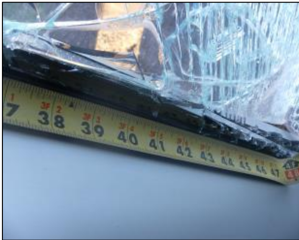
Photo No 178 Post-test, Glazing Tears Specimen 24
