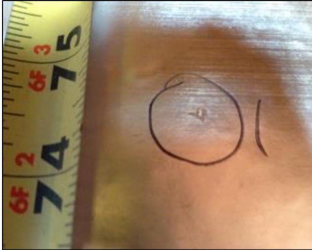
Photo No 46 Post-test, Sliver Perforation Specimen 4
