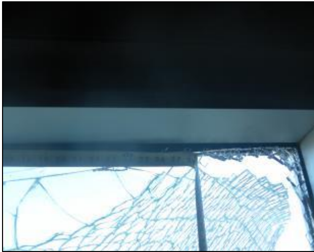
Photo No 176 Post-test, Glazing Tears Specimen 24
