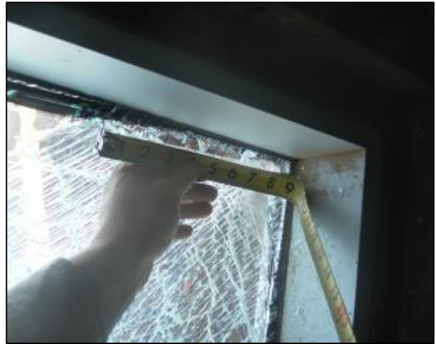
Photo No 181 Post-test, Glazing Tears Specimen 24
