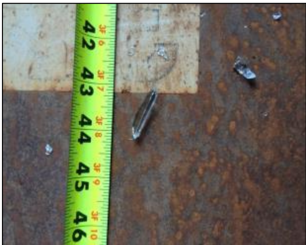
Photo No 13 Post-test, Fragments Specimen 1
