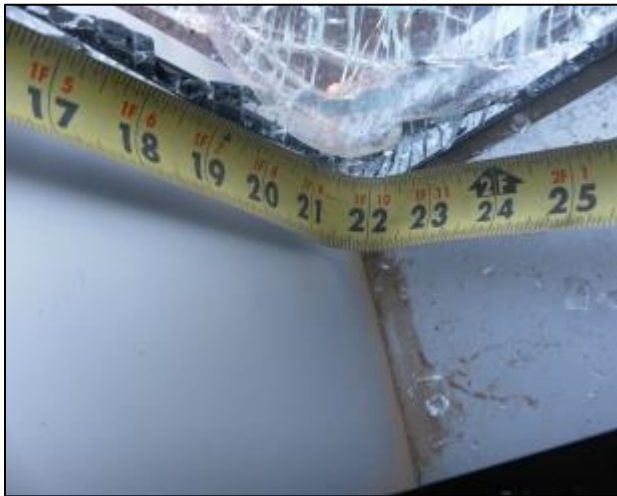
Photo No 182 Post-test, Glazing Tears Specimen 24
